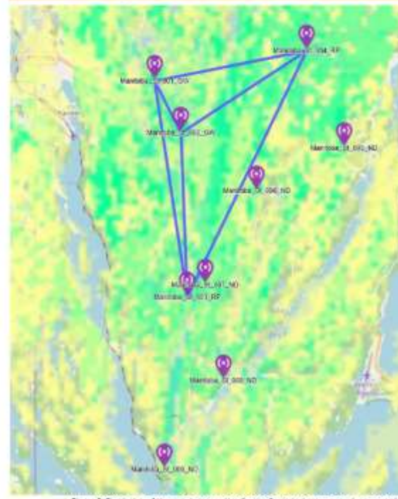
Figure 3: Simulation of the signal propagation for the 4 selected gateway and repeater sites
