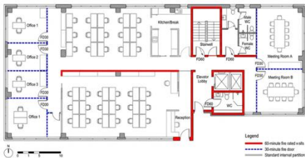
3D Office Visualization: Fire Compartmentation Strategy.
